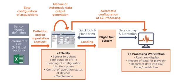
For large Flight Test Systems with many Data Acquisition Units to be managed and an airborne workstation, the eZ Operation software allows seamless and powerful management of the system by automating tasks and summarizing monitoring data in an integrated operator oriented interface. This software can be installed on any PC running Windows 7 or later.
