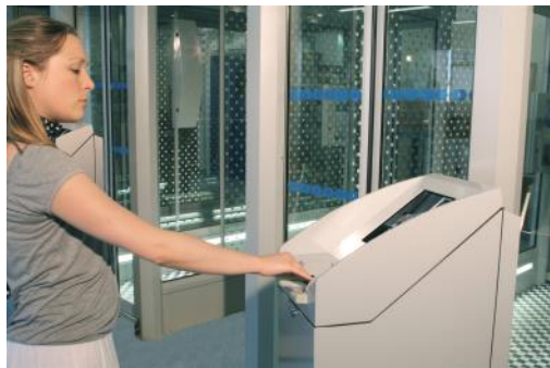
➔ PARAFE France automated border control using fingerprint recognition
