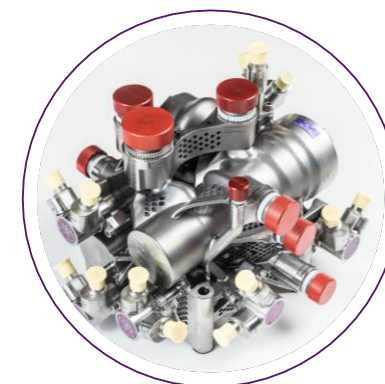
Hydraulic unit for A350 landing gear 50% weight saving
