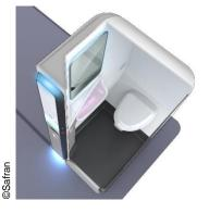
Lavatory. Beacon features anti-microbial materials throughout and deploys 265nm UV light for rapid sanitization of key areas. Functionality of the lavatory is improved by enlarging the washbasin and containing splash contamination. A digital media display in the mirror allows airlines to tailor their own "clean" message to passengers. Moreover, a "clean station" mounted on the outside wall allows passengers to sanitize their hands before or after using the lavatory.
