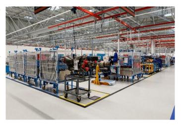
The two workshops benefit from a long-span metal structure that offer great flexibility for the siting of machine tools. They are equipped with skydomes that guarantee natural light levels of 60%.
