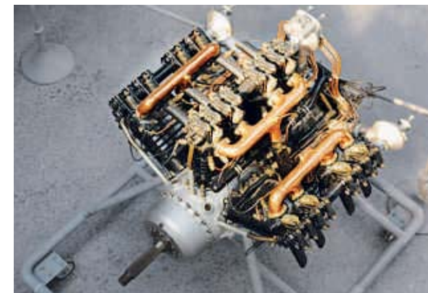
A 450-hp Lorraine-Dietrich 12EB engine, identical to the one that powered the Oiseau-Blanc .
