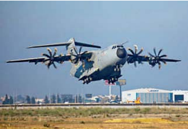
The A400M is powered by four TP400 turboprop engines, each developing 11,000 shaft horsepower.
