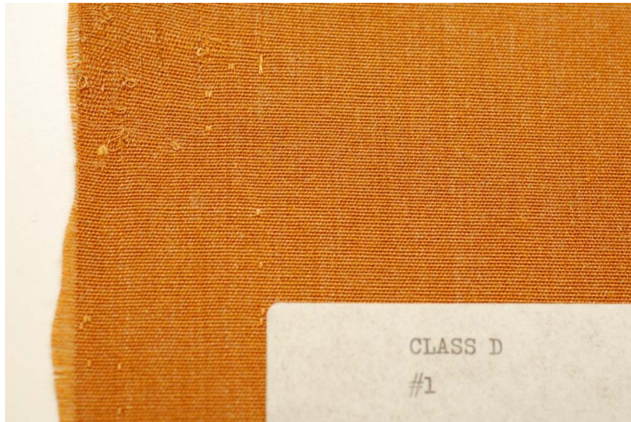
Class D, #1 Floats and loops (acceptable as shown)
