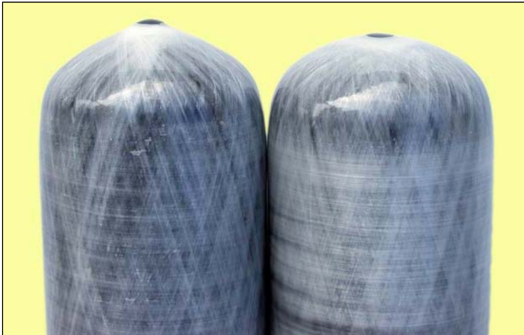
Figure 8: Variations in Shape of Composite Cylinder Bases (acceptable condition)
