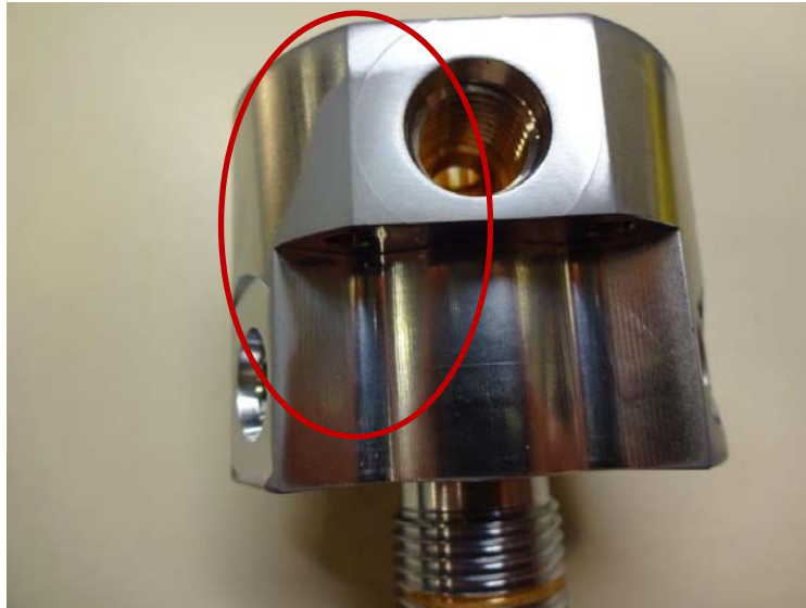
Photograph illustrating: Darkened non-uniform plating
