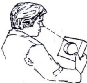
Varying the viewing angle aids in detecting burrs.
