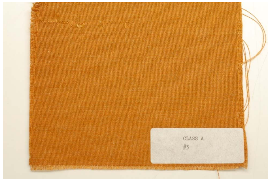
Class A, #3, Floats, bunched or slubs combinations (acceptable as shown)
