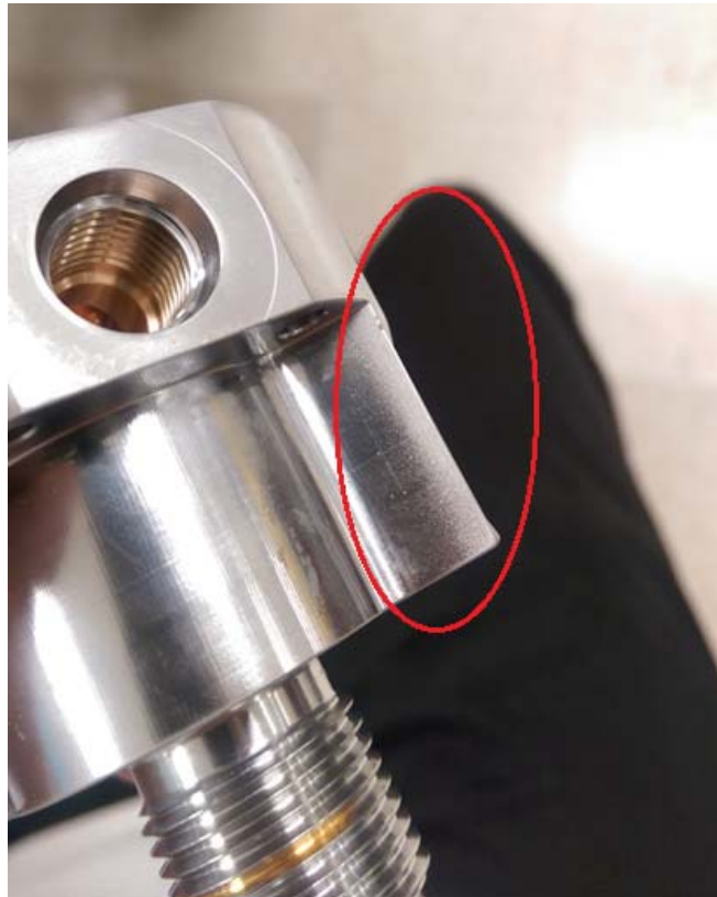
Photograph illustrating: Excessive edge build up
