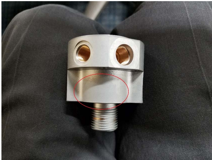
Photograph illustrating: Powdery, non-uniform, and grainy plating
