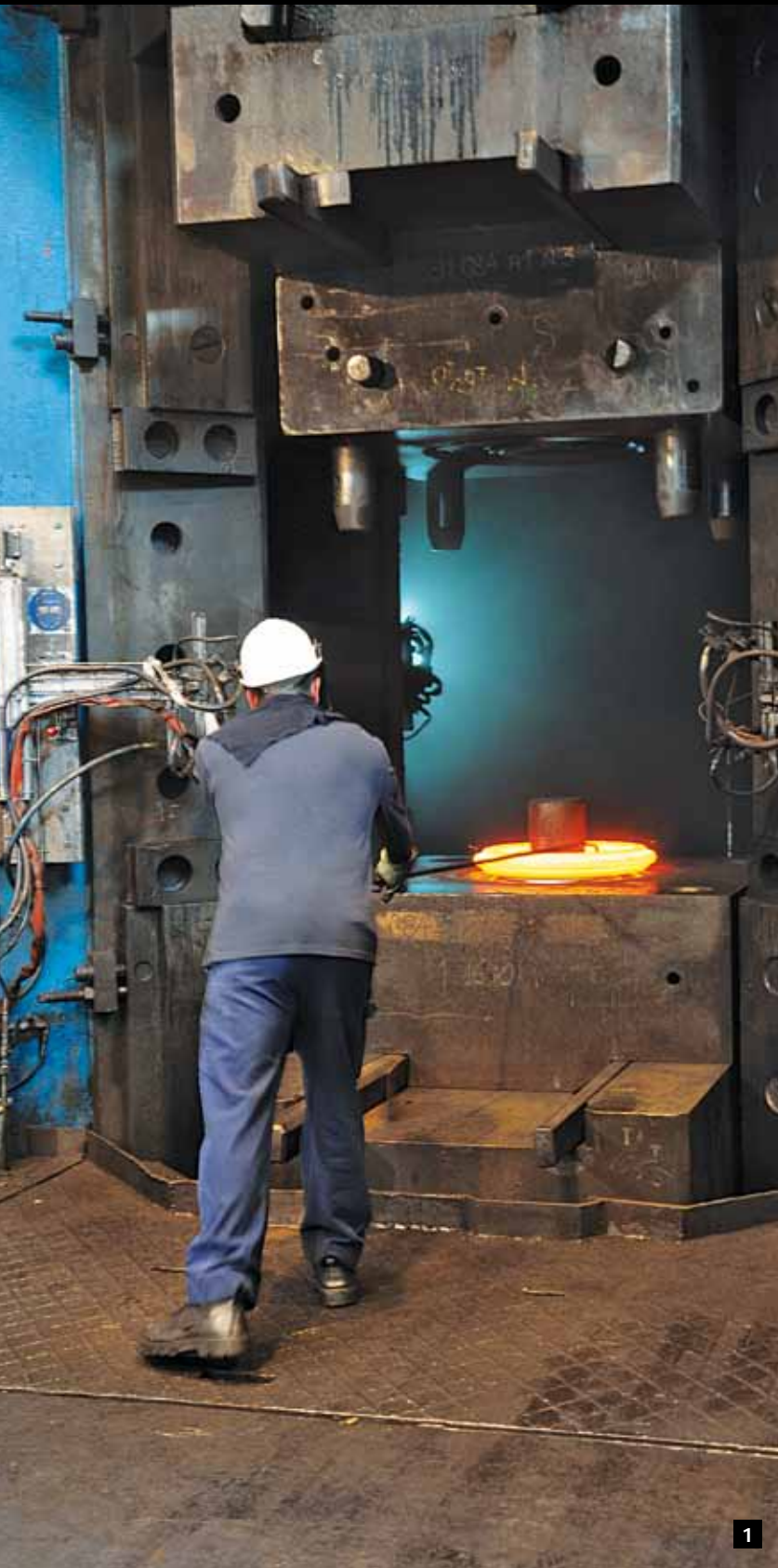
1. 80-TON DROP-HAMMER The part is shaped by the power of this 80-ton drop-hammer.
