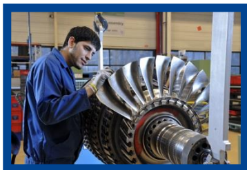
Maintenance of GE90, Saint Quentin en Yvelines, France
