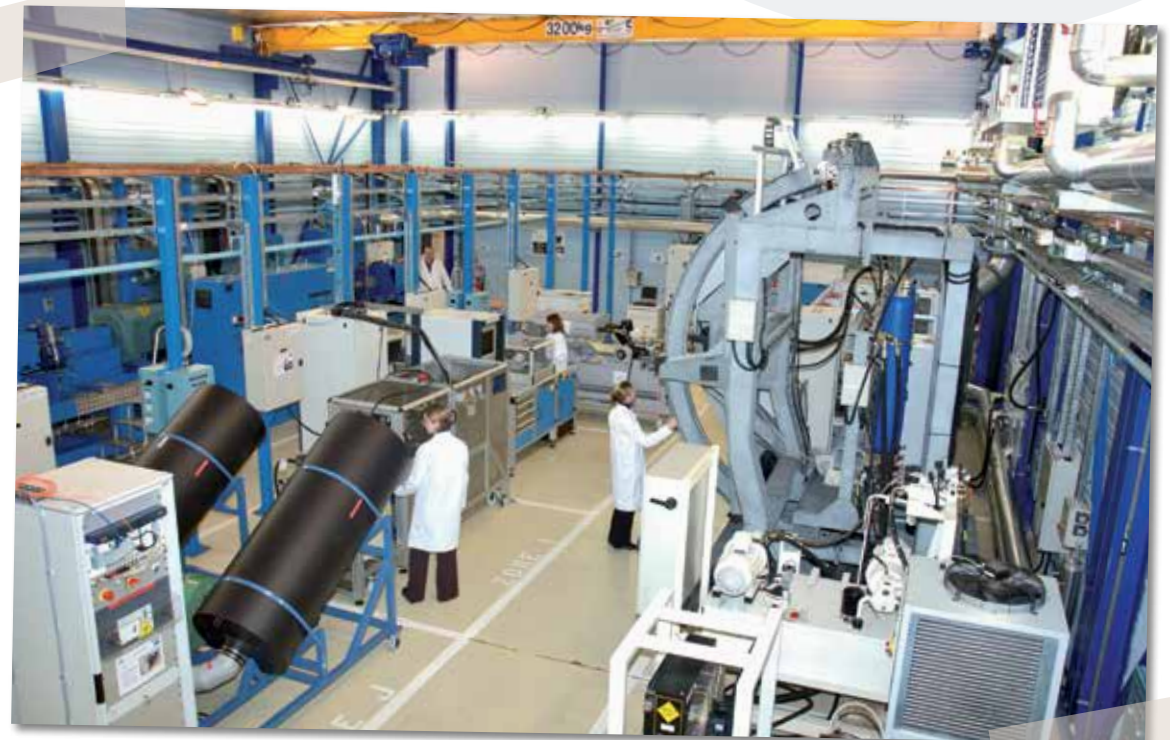
Based in Colombes, near Paris, the Copper Bird® is an exceptional test rig that plays a key role in the development of "more electric" aircraft by Safran and its partners.
