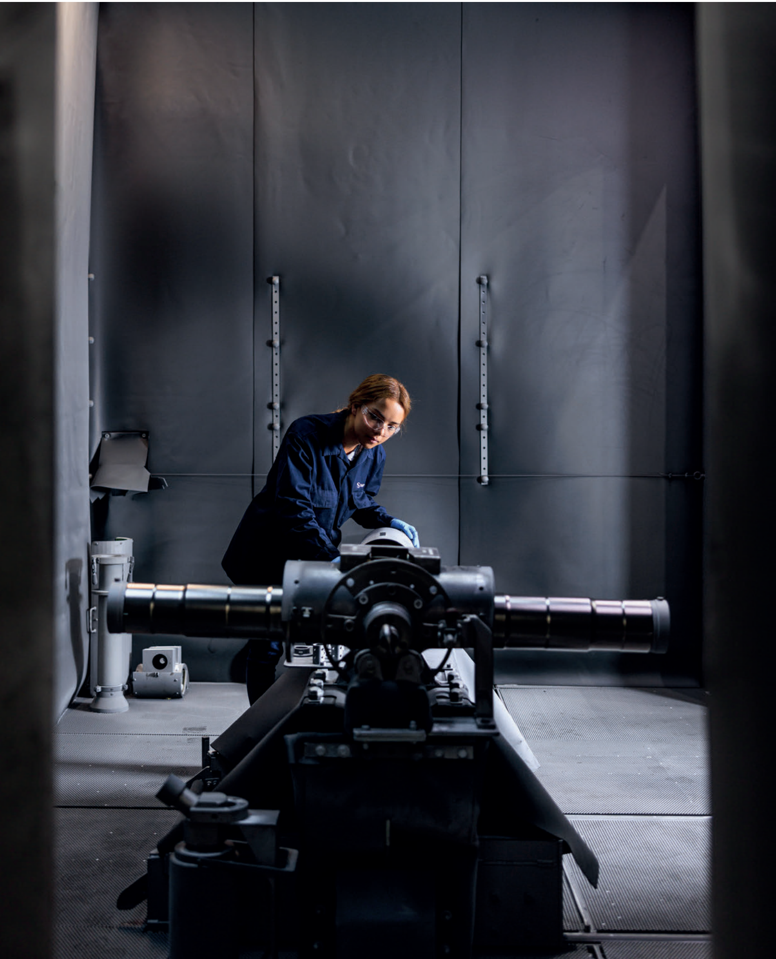
Preparation for a sandblasting operation
