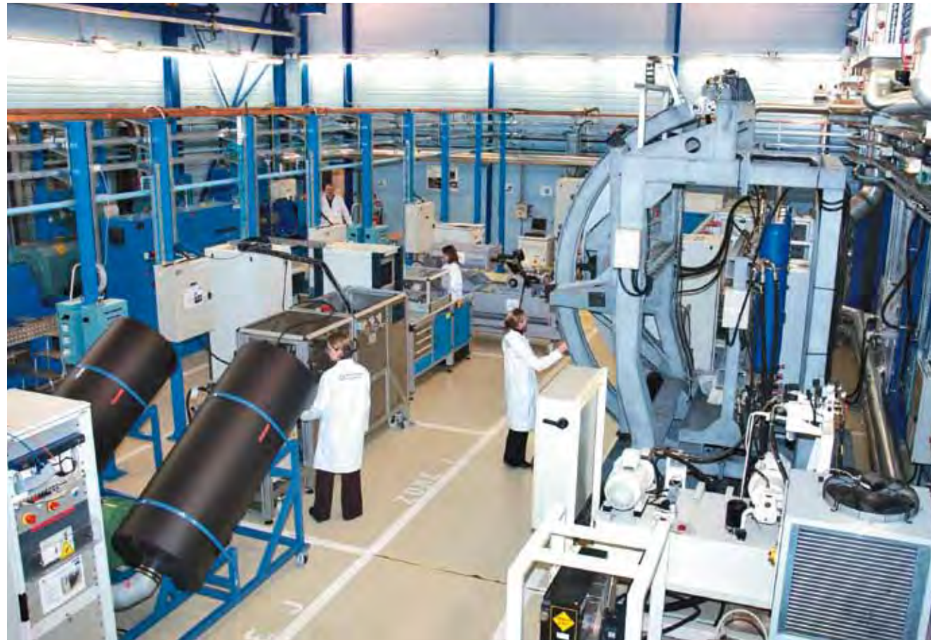
Safran participates in major European research programs working on tomorrow's "more electric" aircraft. The Copper Bird test rig, for example, developed by an Hispano-Suiza-led team for the Power Optimized Aircraft program, is designed to demonstrate the maturity of electrical systems and technologies.
