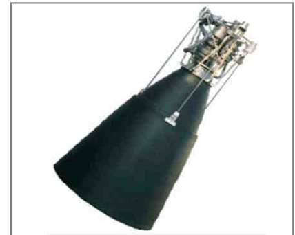
Extendible exit cone for the Vinci motor
